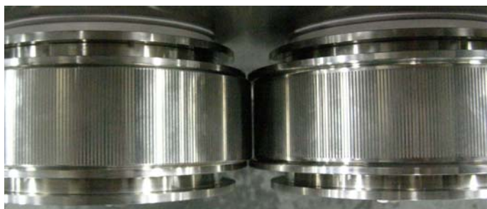
TFC 'Concavo-Convex' Rolls Captures Product in Compaction Zone
