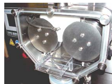
Optional Vacuum Assisted Deaeration at the Compaction Zone
